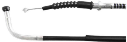
MMCB009 CABO EMBREAGEM YAMAHA: FACTOR 125 YBR E (2009-2016) / FACTOR 125 YBR ED (2009-2010) / FACTOR 125 YBR K (2009-2016) / FACTOR 125 YBR K1 (2014-2016)
